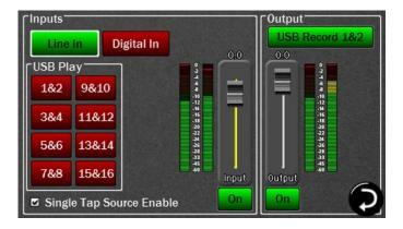
The engineer likes this set up and has a second guitar player coming in the next day for more overdubs. To save this scene (including routing and levels), click on the TOOLS icon on the bottom, bush the Save Scene button, push Scene 1. To recall the setting, push the Recall Scene
