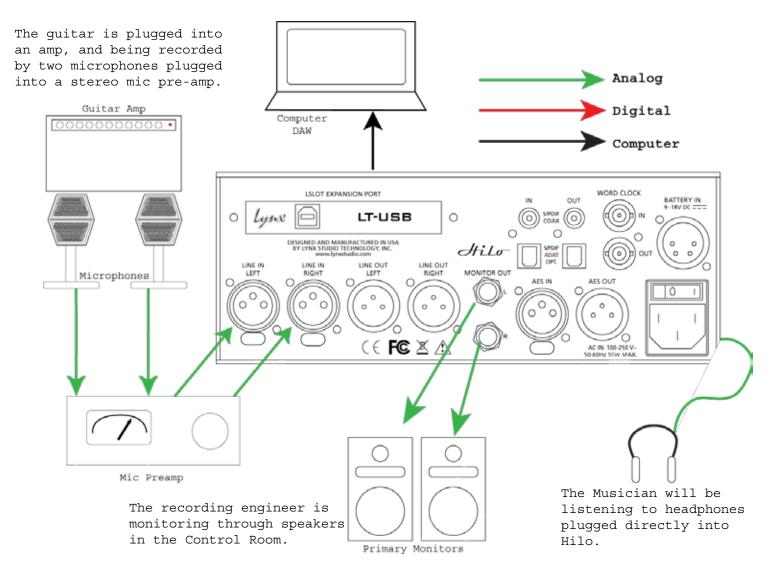
The cable connections: Monitor Out > Speakers in Control room Headphone Out > Phones on musician Line In > Signal from stereo mic preamp USB > Recording computer (alternatively we could do this as going to an AES16e card) Set up the Busses in DAW organized as: Play 1+2 = DrumsPlay 3+4 = GuitarsPlay 5+6 = Bass and Keys Play 7+8 = Vocals
