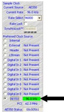
If the Sample Rate listed has a RED background, or the box displays “Not Present”, then there is a problem with the AES50 connection. Double-check cable connections and device settings.
