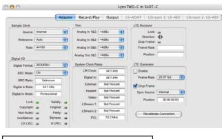
**Analog Trim**: Sets nominal Input and Output levels to either +4dBu or -10dBv.
