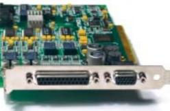
The Lynx Two's audio I/O reaches the card through breakout cables attached to these two D-type ports.
