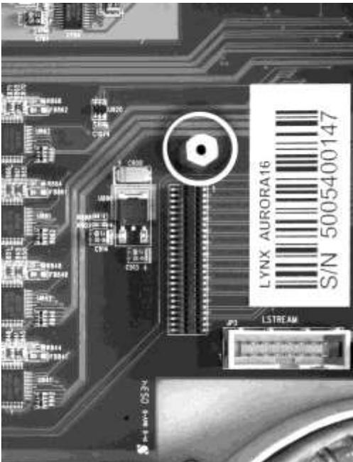
6. Grounding yourself to earth ground, remove the LT-TB from its protective anti-static bag.
